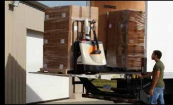
Thousands of applications without receiving/shipping docks require delivery from truck to curb side via lift gates. Crown's compact design, exceptional maneuverability and brake override features make the WP 3000 Series ideal for these applications.
