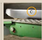
Uniquely designed to protect the forks, the riser axle on the WP 3000 Series is located at the highest point possible. This eliminates frequent repairs required when the riser axle is damaged by constant contact with dock boards, pallets and uneven floors.
