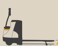
Lift cutout at full lift protects the motor from continuing to work once full lift is reached. This reduces energy consumption and extends component life.
