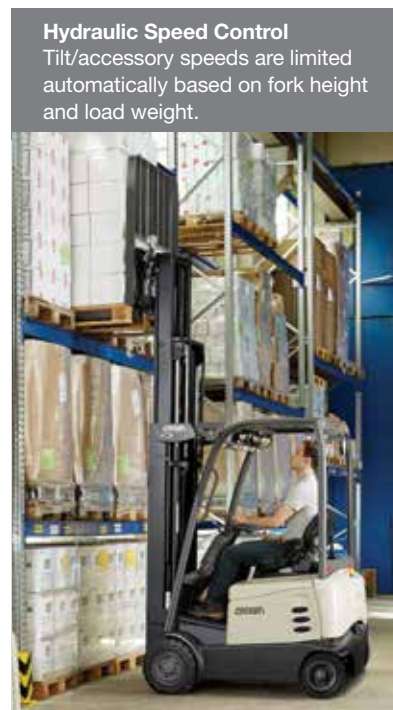
Travel and Cornering Speed Control The on-board intelligence assists the operator with control based on load weight, lift height, steer angle and truck speed.
