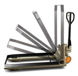
**Skid Adapter** increases lowered height to 5.5 inches to permit skid handling. Raised height increases to 10.5 inches. Adapter latches in vertical position for pallet-handling tasks.
